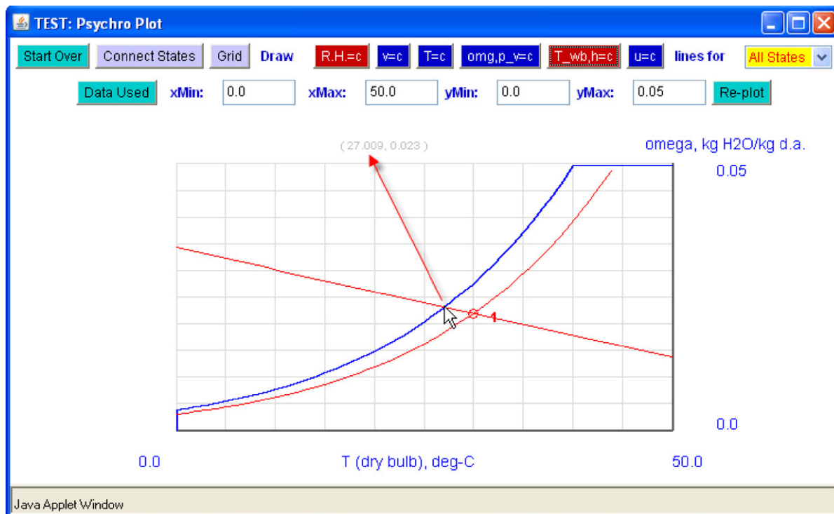
Fig. 11. As in any thermodynamic plot, constant property lines can be drawn on a psychrometric plot. In this figure, the wet bulb temperature for state-1 computed in Fig. 10 can be deduced by parking the pointer over the intersection of the constant T_{wb} line and the saturation line (shown by the arrow).
